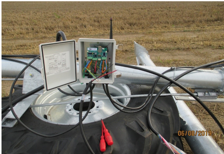
Figure 19 wireless node mounted
