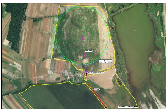
Figure 7 - 2D planning Indicating needed supply pipe
