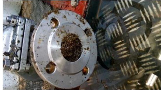
Figure 5. Left is caked solids blocking the check valve with swing-flap removed, right is a modulation valve caked with solids.
