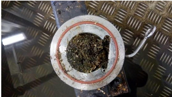
Figure 5. Left is caked solids blocking the check valve with swing-flap removed, right is a modulation valve caked with solids.
